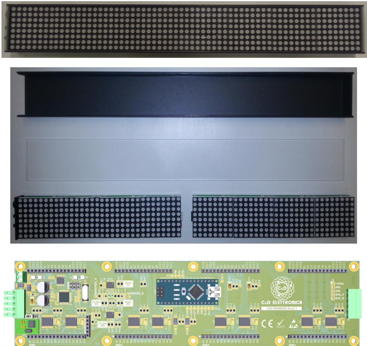
Fig. 3. Cased 2-cell FlashMat display, with an Arduino Nano master board (optional) installed on one of the cells.
