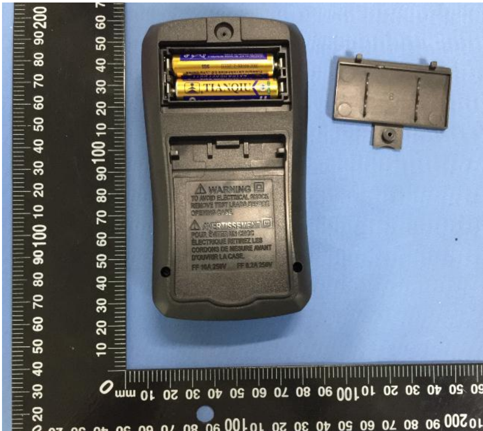
Photo 8 – Battery compartment view
