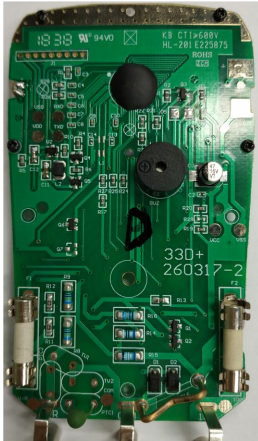
Photo 15- Internal view of UT131D
