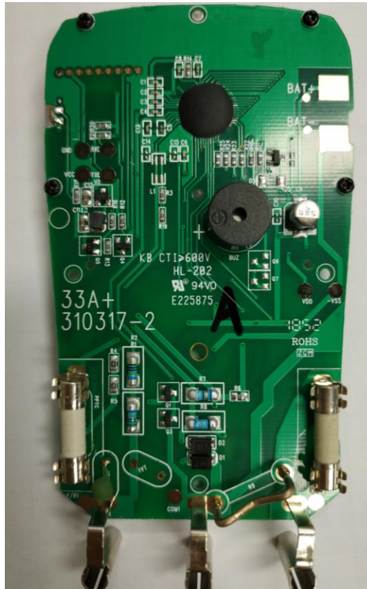
Photo 9 – Internal view of UT131A
