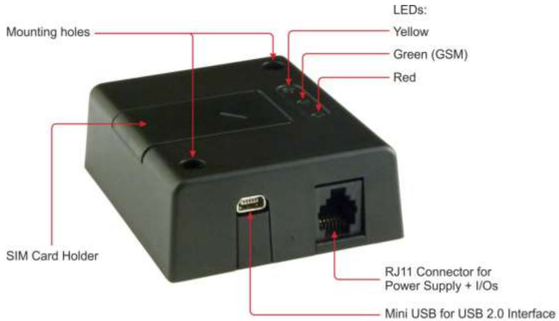
Figure 1: Connector on rear side of the Terminal
