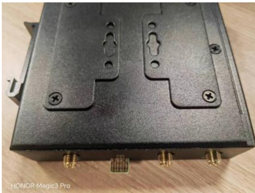
Fig. 9 Install the sim card
