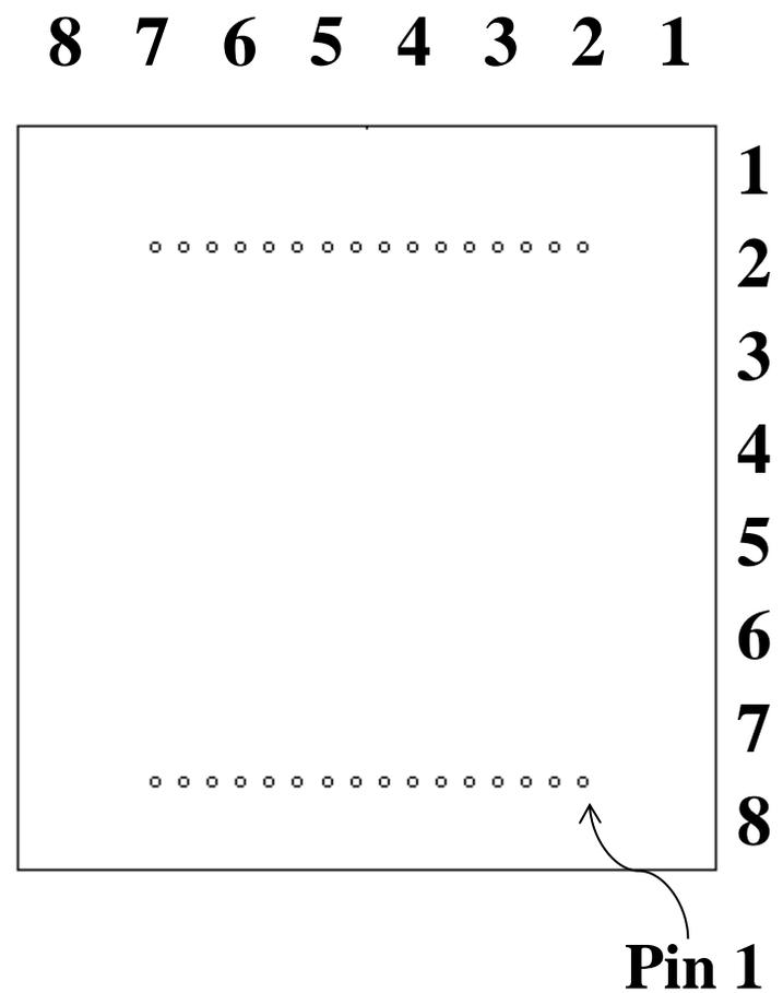
If possible, on this side print a dot near the pin #1, to identify it.
