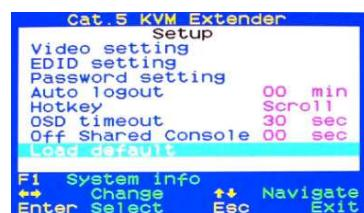
copy the factory default monitor DDC data to both the Transmitter and Receiver Units.
