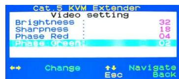
and green so that you don't have any coloured edges on the right or left of any white and black fields or vertical lines or so that red and green vertical lines are **exactly in the same line with blue vertical lines** on the test picture. Then adjust brightness and sharpness using the Windows desktop icon texts and also open text windows with text until you are satisfied. You may have to go through the complete procedure several times. Changes have to be stored when leaving the OSD!
