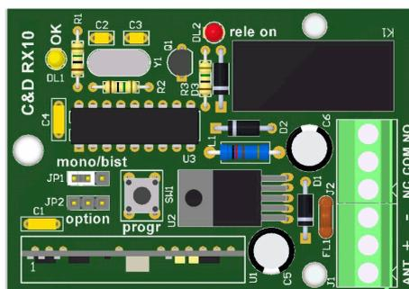
**Ricevitore RF 1Ch 434MHz C&D RX10**
