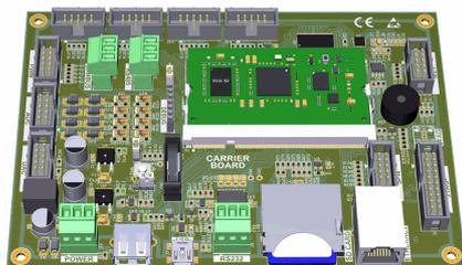
Ethernet 10/100 Mbps Ethernet (based on Microchip LAN8742AI Ethernet PHY)
